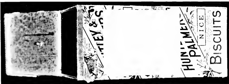
FIG. 47.—A SIMPLE FORM OF MOSQUITO TRAP MADE OUT OF BISCUIT TINS, THE INTERIOR OF WHICH HAS BEEN BLACKENED. [Face page 242.]
